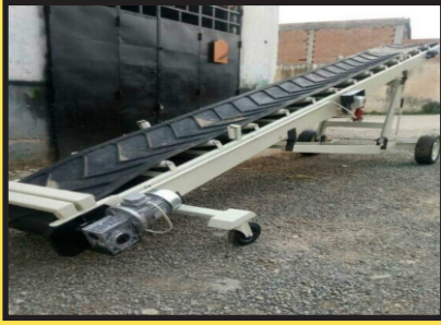
Chevron Loading Conveyor
