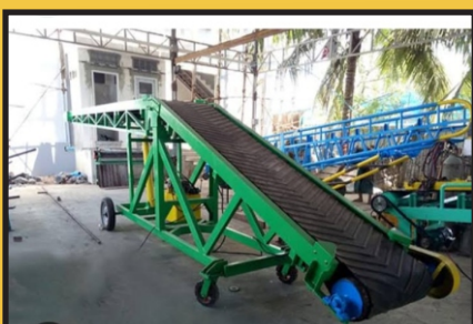
Truck Loading Conveyor
